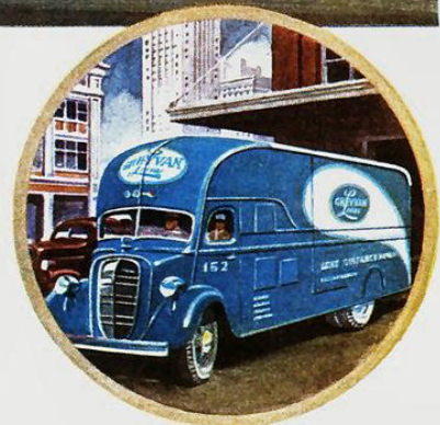
Studebaker Cab-Forward efficiency is most evident in cramped quarters, where the saving of upward of 40 inches in overall length saves hundreds of minutes and gallons of fuel in daily maneuvering.
